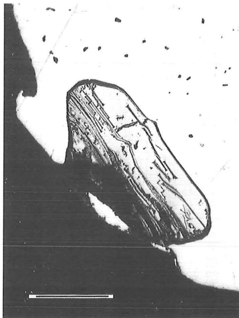
Fig. 5. Polished section of a platinum grain (light grey), including luberoite (dark grey). The latter, located at the border of the platinum, displays cleavages filled with anatase. Reflecting light microscope, unpolarized light, oil immersion. Scale bar = 100 \mu\text{m} .
